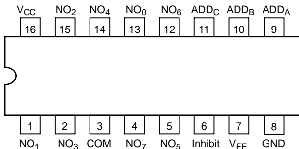
Figure 1. Pin Connection (Top View)
